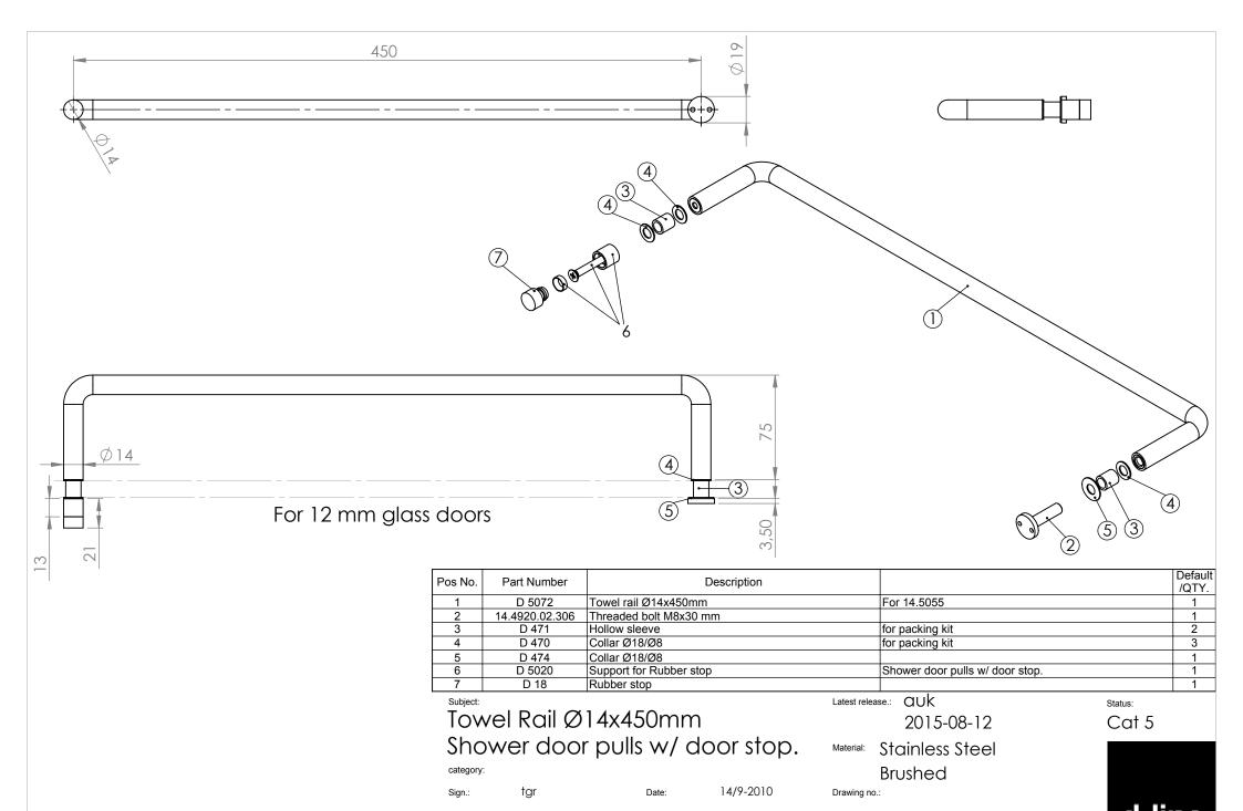
Dimension without tolerance, follows DS/ISO 2768-mK. This drawing is the property of d line a/s, and is not to be copied or shown to third parties.
